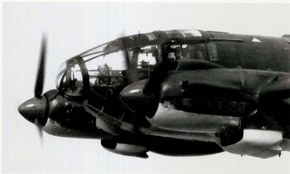
ABOVE: In this close-up of an He 111 H the front gunner is clearly visible lying in the fuselage nose with the pilot behind. The photograph also shows the yellow '87' octane triangle painted above and behind the cockpit canopy.
