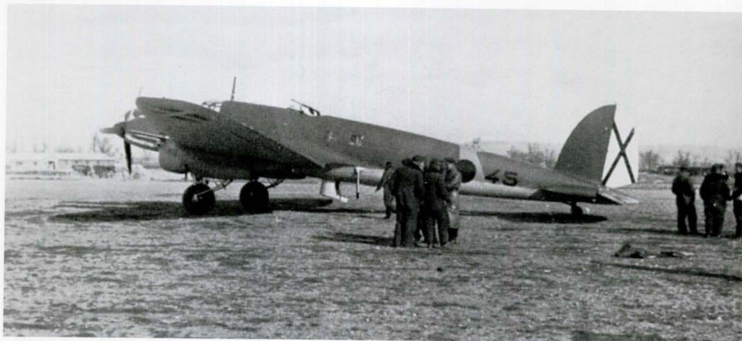
BELOW: Early in 1938 the first He 111 Es were delivered to 2.K/88. This variant could carry a 2,000 kg (4,400 lb) bomb load and was powered by the more powerful Jumo 211 D engines. This aircraft, 25●45, retains the pre-war three colour camouflage carried by the Luftwaffe with its spinners painted in the Staffel colour, red.
