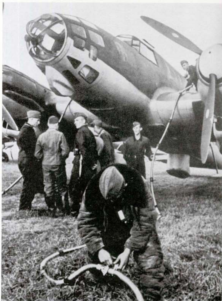
RIGHT: Ground personnel connect fuel hoses to an underground storage tank in preparation to re-fuel this He 111 F-4. Note the 7.9 mm MG 15 has been removed from the spherical mounting in the glazed nose and the retractable ventral 7.9 mm MG 15 'dustbin' in the extended position.
