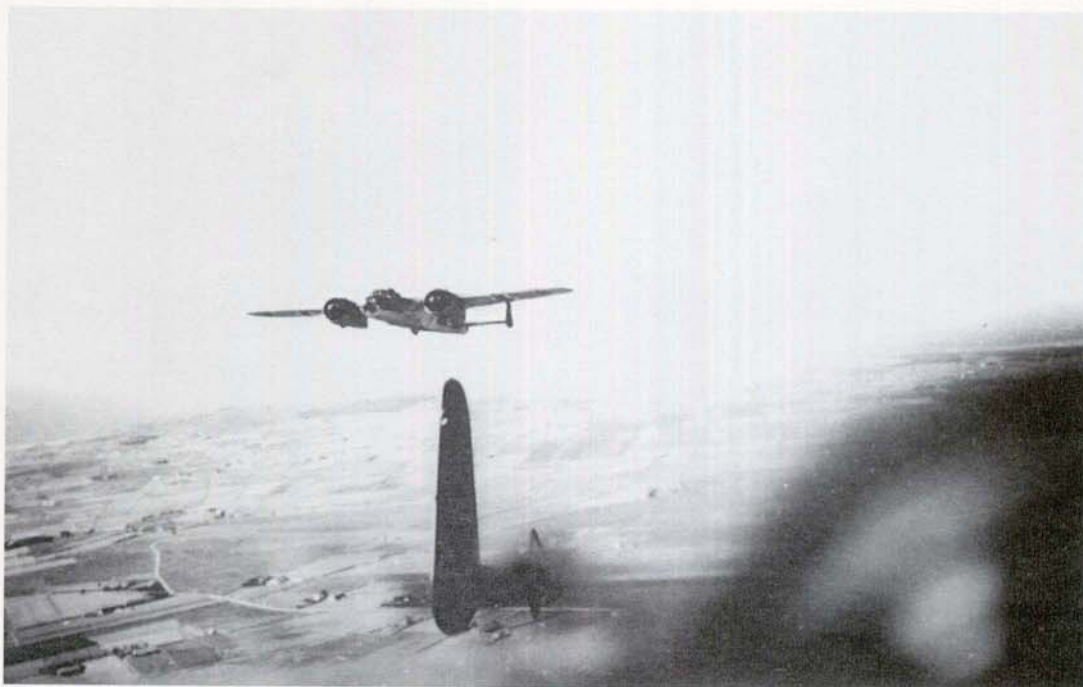
LEFT: A rare in flight photograph of a Do 17 M-1 bomber over Germany. It gives an excellent idea of the dividing line between the dark green upper and pale blue lower surface camouflage.
