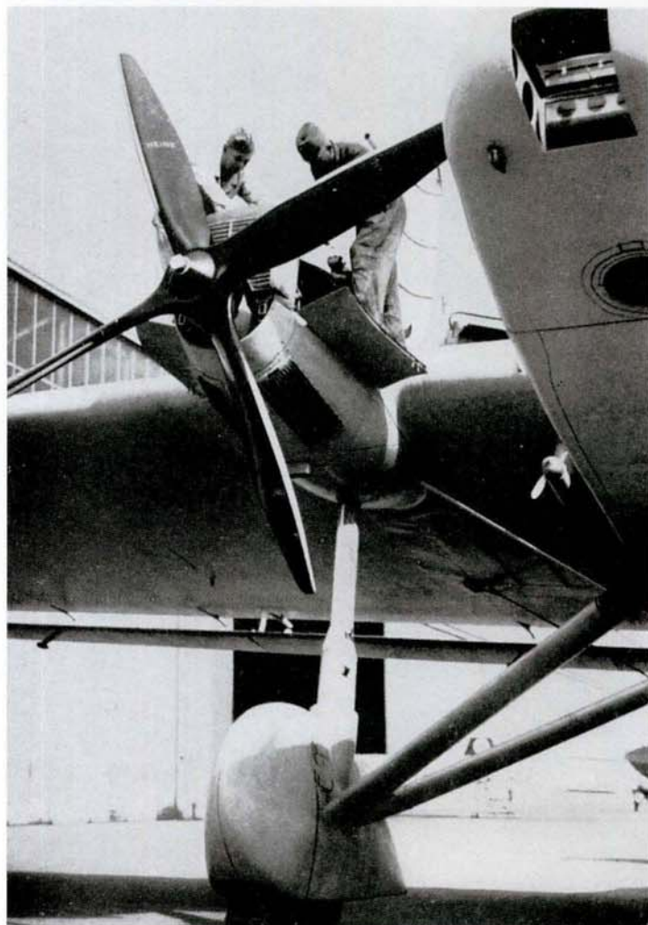
ABOVE: Mechanics at work on the starboard 750 hp BMW VI engine of a Do 23. The somewhat clumsy fixed, spatted undercarriage is notable as is the four bladed wooden propeller and generator mounted under the wing centre section near the fuselage.
