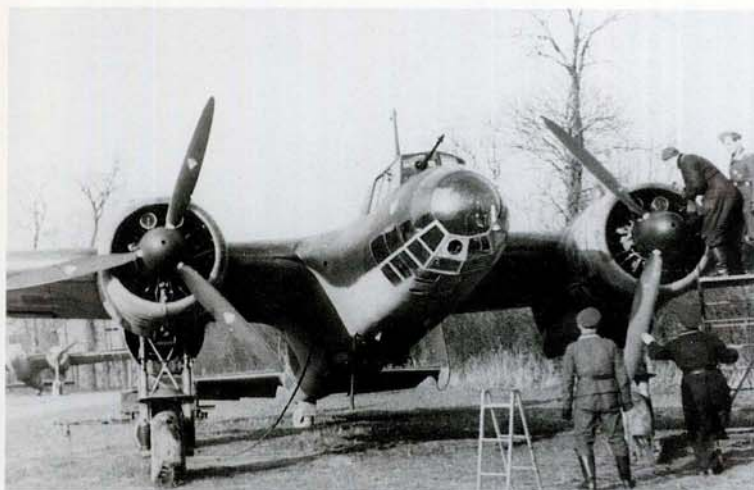
ABOVE: The soft-edged camouflage dividing line is shown well on this photograph of mechanics at work on the port radial engine of a Do 17. Note the black and white triangular logos of the VDM company painted on the starboard black green colour propeller blades.
