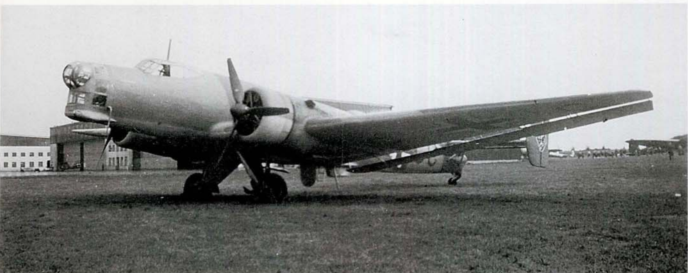
BELOW: Because of the problem with the Jumo 205 Diesel engines fitted to the Ju 86 D, these were replaced with two 850 hp BMW 132 F radial engines, a licence-built version of the American Pratt and Whitney Hornet.
