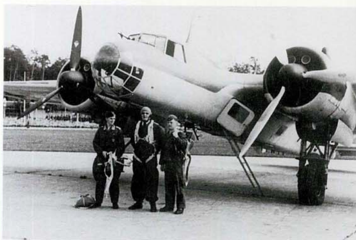
ABOVE: Note the difference between the propellers on this Do 17 M. It is evident that the port propeller has been changed since the blades are in natural silver while the starboard propeller is in the standard black green finish with the VDM manufacturer's logo.
