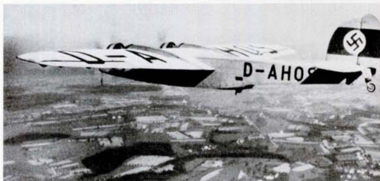
ABOVE: The Do 11 was the first European bomber to be fitted with a retractable undercarriage but because of its unreliability relatively few were delivered to the Luftwaffe before the type was replaced by the similar Do 23 with conventional fixed gear and different engines. The Do 11 D seen here with the civil registration D-AHOS, had a new shorter span wing with redesigned wingtips. It was delivered in small numbers to I./KG 154 and I./KG 553 before it was replaced by the Do 23.
